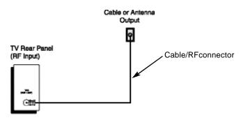
1) Connect an RF Cable from the wall outlet into the RFCable In on the back of the TV.
